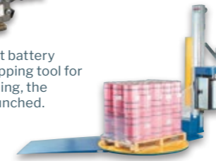
1999 Introduction of the FS-series Pallet Stretch Wrapping Machines, which featured an ultra-low turntable, a revolutionary 400%, 2-motor Power Pre-stretch film carriage.
